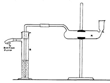
perfectly dry it is again attached to (B) and completely submerged to the neck of the funnel (c) in a sand bath. The suction is now connected to (B), which contains approximately normal sodium hydroxide and the temperature of the sand raised slowly to 145°. It is kept at this temperature for a few minutes, and finally brought up to 260°. The benzoic acid is thus sublimed and then retained in (B) as sodium benzoate.
